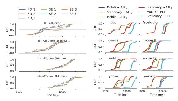
**Fig. 5.** The distribution: (1) the ATF time of the websites under mobility condition across different operators, and (2) The ATF time and PLT of the websites under different mobility conditions.
