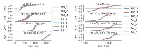
**Fig. 3.** The distribution of (1) DNS lookup time, TCP connect time, TTFB, and PLT and (2) ATF time as approximated using the two approaches.
